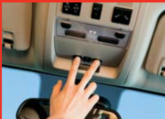
Typical UHR located in overhead console.
